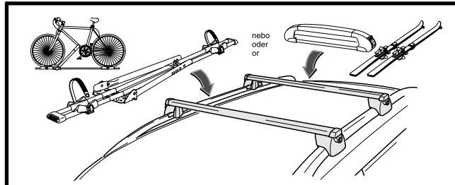
**Caution.** We recommend only using sockets mounted on the T-slots (using a T-bolt). Assembly with metal U-shaped sockets could damage the surface treatment on the bearing profiles of the cross rail.
